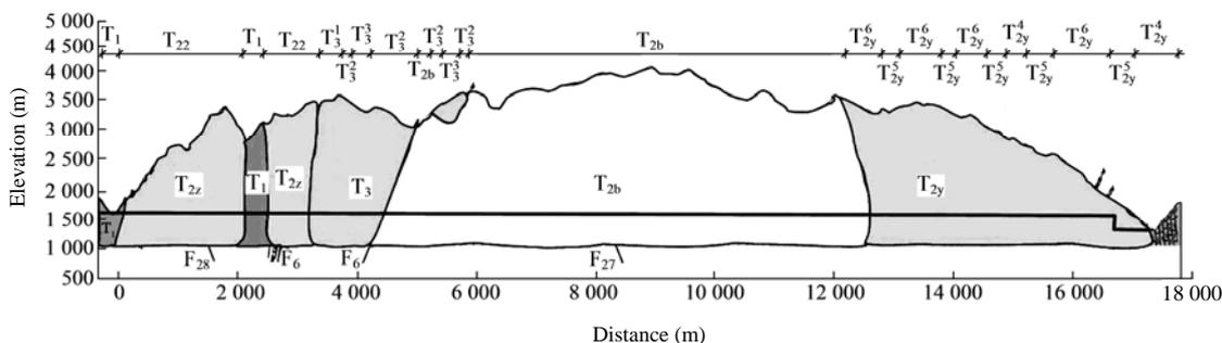
**Fig.2** Geological profile along the diversion tunnels.
