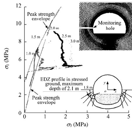
**Fig.9** Measured EDZ profile on the headrace tunnel section and numerical calibration (the overburden depth is about 1 733 m).
