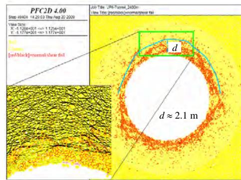
**Fig.10** EDZ profile simulated by PFC (the overburden is 1 500 m).
