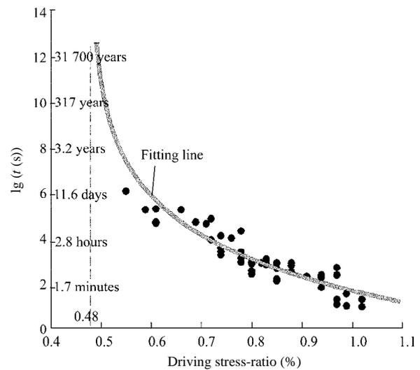
**Fig.7** Static-fatigue test data for marble group T<sub>2y</sub><sup>5</sup> with exponential fitting.
