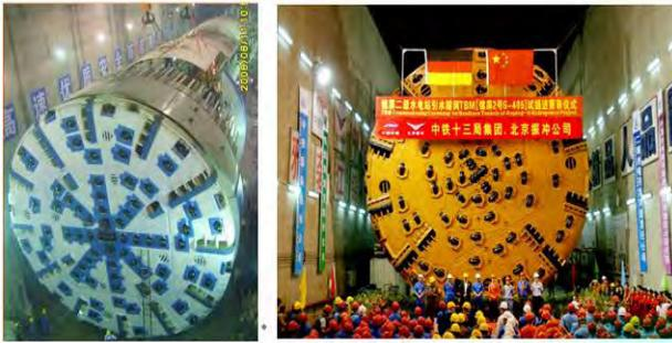
**Fig.2** TBMs used in tunnel excavation (the left one is Robins TBM for the headrace tunnel No.1 and the right one is Herrenknecht TBM for the headrace tunnel No.2).
