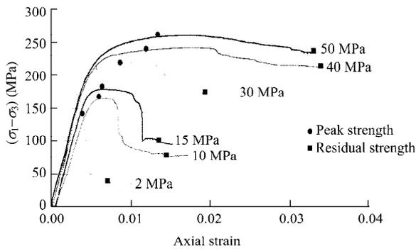
**Fig.6** Results of triaxial test for marble T<sub>2b</sub> in Jinping II project.
