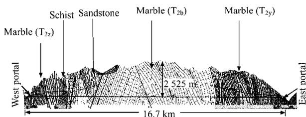
**Fig.3** Simplified geological profile along the headrace tunnel No.1.
