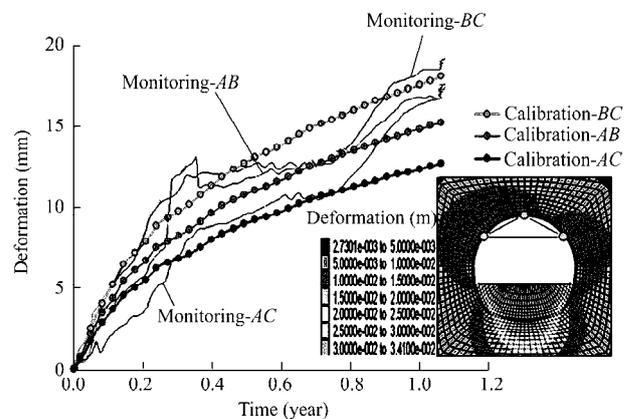
Fig.11 Measured deformations of ground and numerical simulated results for tunnel section KP(1)1+675.
