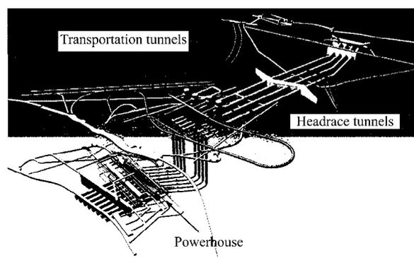
Fig.1 Layout of main hydraulic facilities of Jinping II project.
