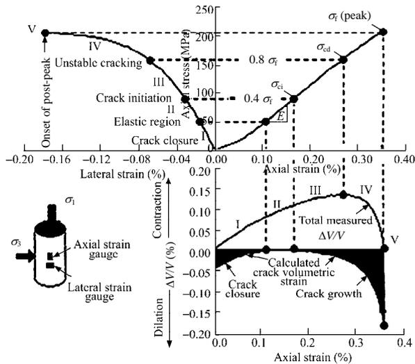
**Fig.4** Stress-strain curves obtained from a single uniaxial compression test on Lac du Bonnet granite [4].
