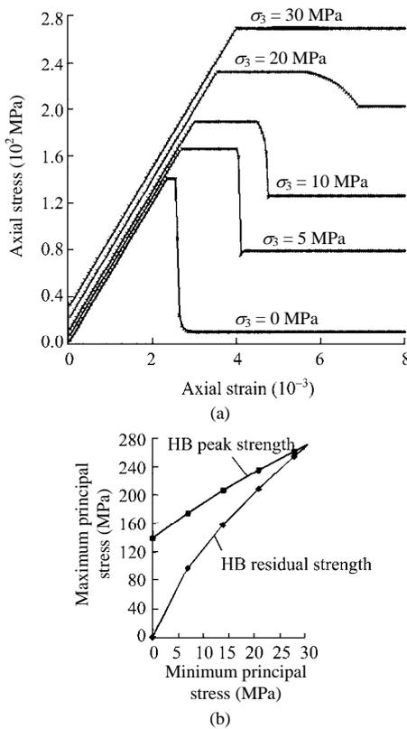
**Fig.8** Description of marble brittle-ductile-plastic transition behavior with different confining pressures.
